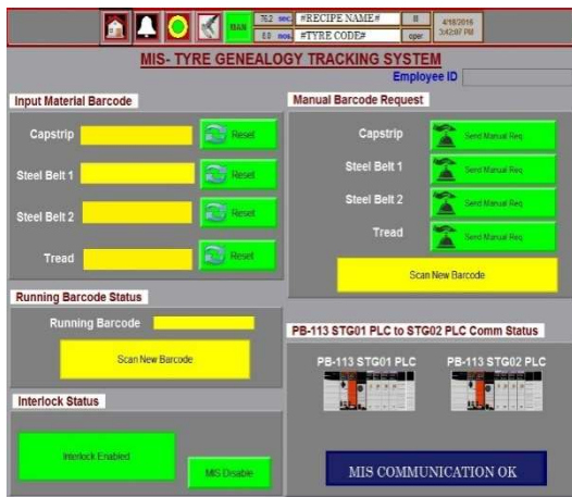
Fig. 8 HMI screen for MIS communication
